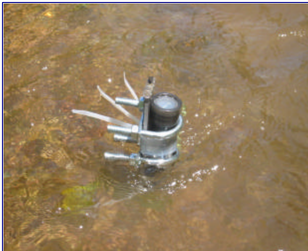
Figure 13. Close up view of deployed HOBOTM Water Temp Pro automated temperature sensor.
